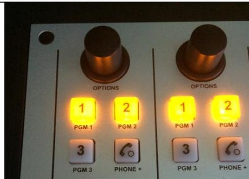
On the Axia the Options knob located at the top of each channel will adjust Trim by default.
