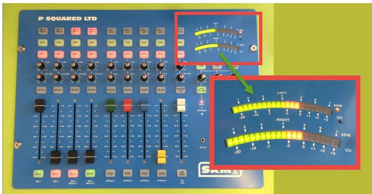
The meter is located on the top of the ARC8 and Axia iQ mixers.
