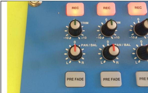
On the SRM the Trim knobs are located just below the REC buttons on each channel.
