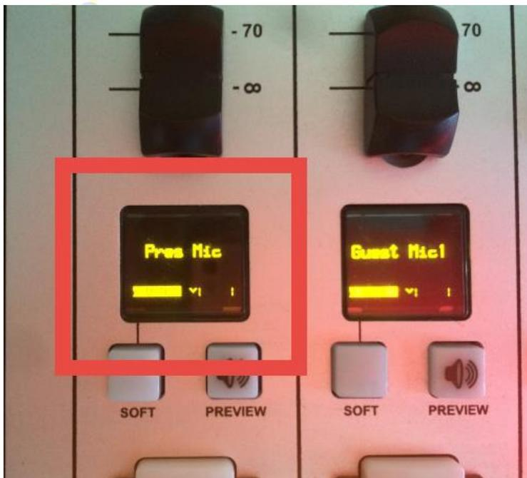
The Axia iQ fader channels are assignable on the fly which means the microphone channels could be on any of the faders. The default is on the left hand side of the mixer but you will need to look at the channel assignment screen on each channel to find the fader(s) you want.
